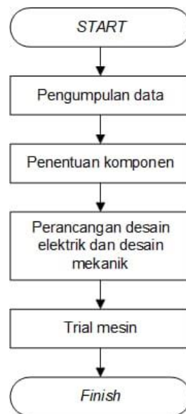
Gambar 1. Flowchart Proses Retrofit CNC Milling MAHO MH 600E
